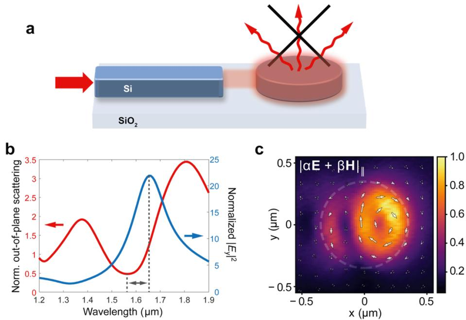
**Figure | Decoupling of anapole condition and near-field energy maximum in on-chip excitation of high-index nanodisks.**
