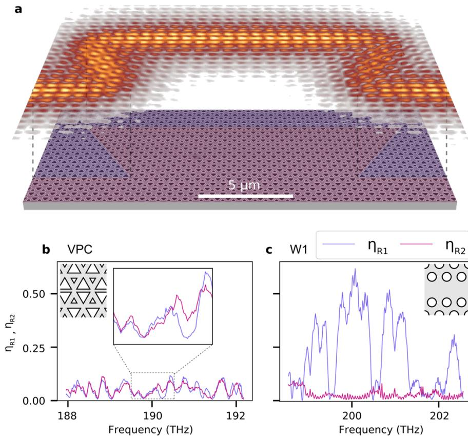
**Figure | Experimental visualization and quantification of robustness in a valley photonic crystal.**
